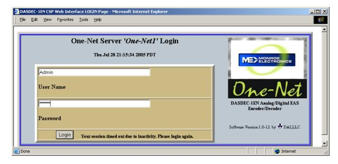
Type "Admin" (no quotes) as the default user name, and "dasdec" (again, without quotes) as the password. Press the left mouse button over the <u>Login</u> button. With the correct user name and password, the One-Net will login. If the user or password is incorrect, the One-Net will display a message indicating the problem. If the One-Net is left unattended for 10 minutes, it will automatically logout. A message indicating session timeout will be displayed on the login screen.
