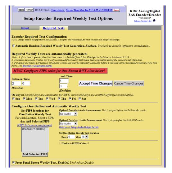
Click on the FIPS code from the list for the County where the unit is installed and Click on the Add Selected FIPS button. This county will be used in the Automatic Weekly test Message. The following display will be shown.
